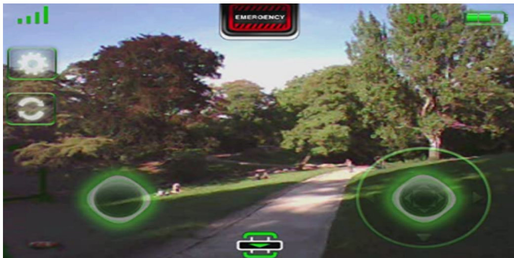
Figure 3.11.2: Augmented reality vision based drone control
