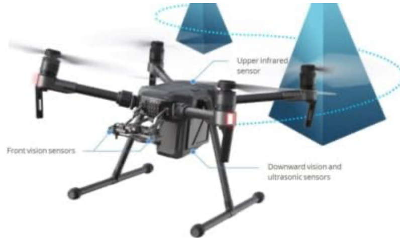
Figure 5.5.1 An example of infrared sensor being used to avoid obstacles
